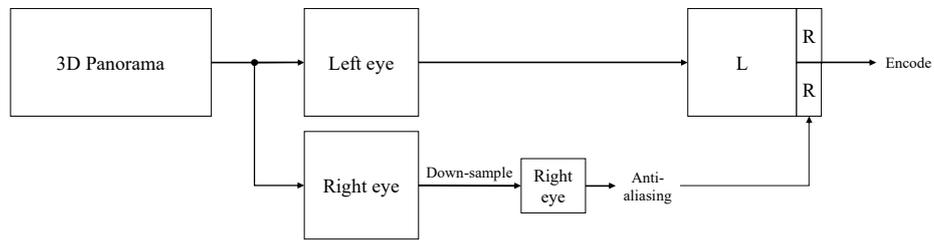
**Fig. 1.** Framework of asymmetric splicing method for 3D panoramic image
