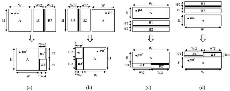
**Fig. 3.** (a), (b) Splicing method for side-by-side. (c), (d) Splicing method for top-and-bottom
