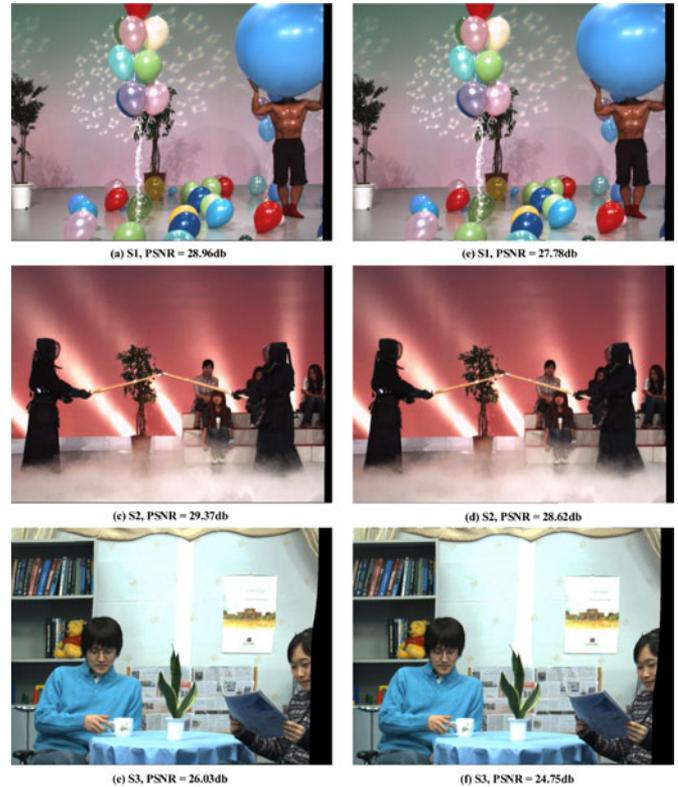
Fig. 9. Synthesized views. (a), (c), and (e) were obtained using the original IDW method, and (b), (d), and (f) were obtained using our proposed method.
