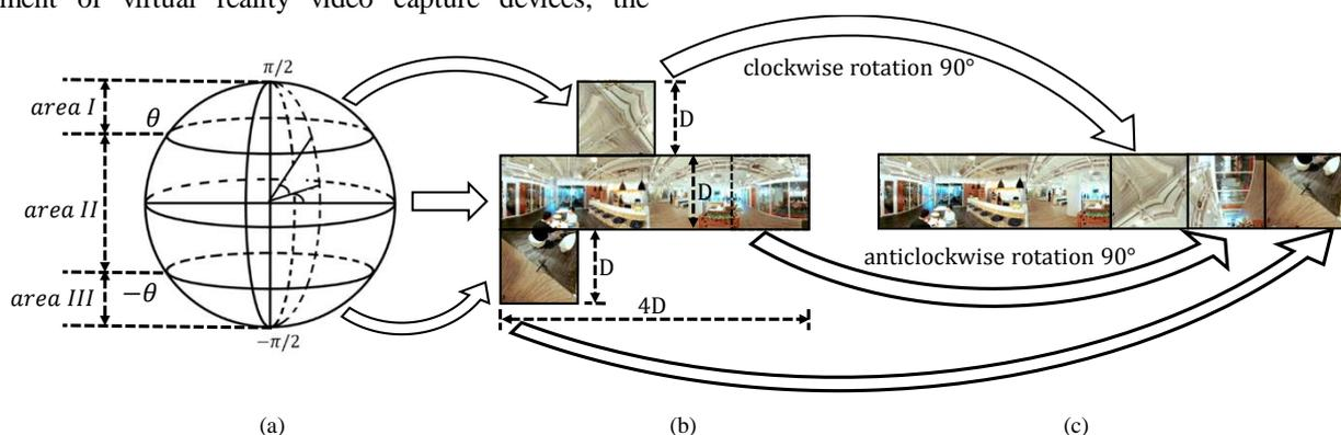
Fig.1 The schematic diagram of our proposed projection method in this paper
