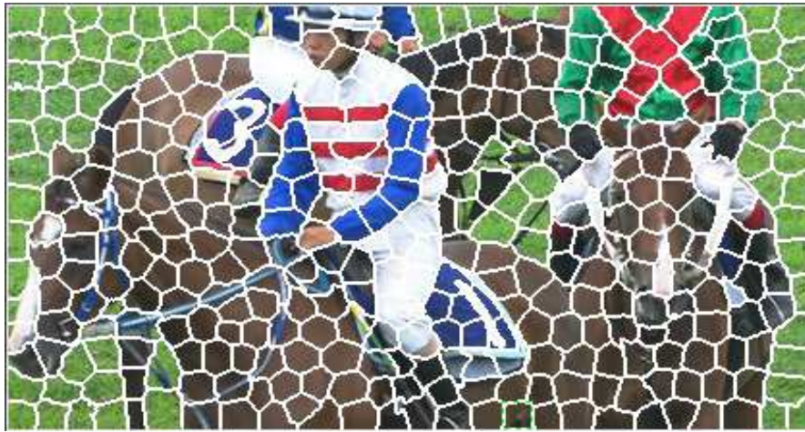
Figure 1. "Racehorse" image segmented into superpixels of size 256 pixels with SLIC
