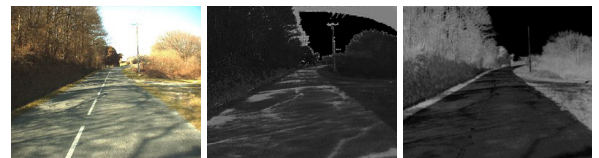
Fig. 1. Raw image of a shadowy road (left) and its H (middle), S' (right) components.
