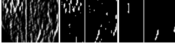
Fig. 6. Lane marking feature extraction. Left: filtered image. Middle: binarization. Right: small isolated regions removed.
