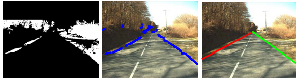
Fig. 2. Road boundary modeling. Left: segmentation result. Middle: extracted boundary points. Right: detected road boundaries.
