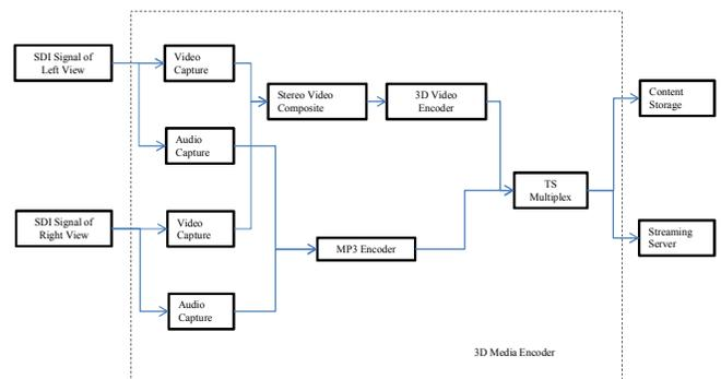
Fig. 2. Proposed architecture of 3D media encoder
