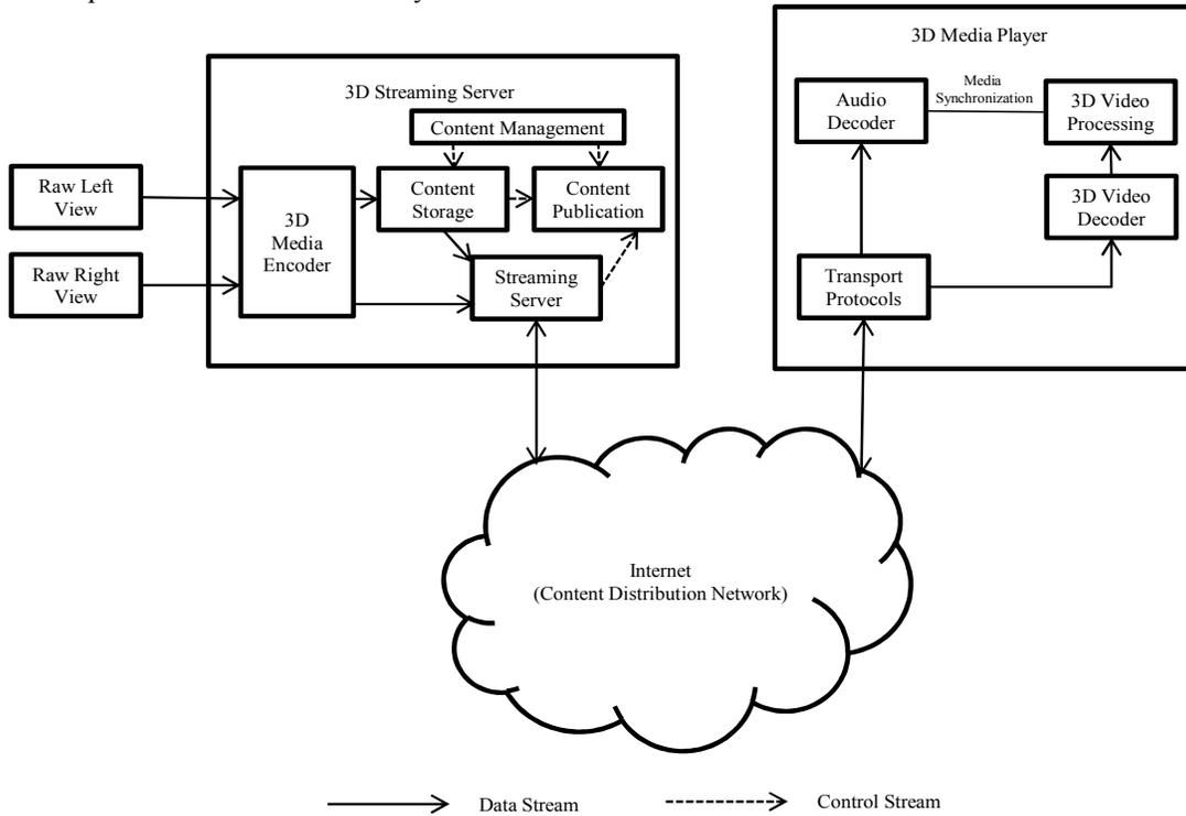
Fig. 1. Proposed architecture for 3D streaming system
