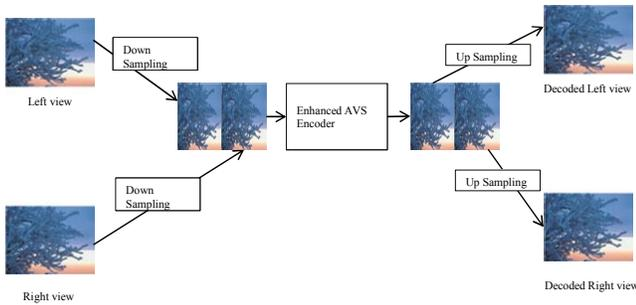
Fig.3. Proposed 3D video codec architecture
