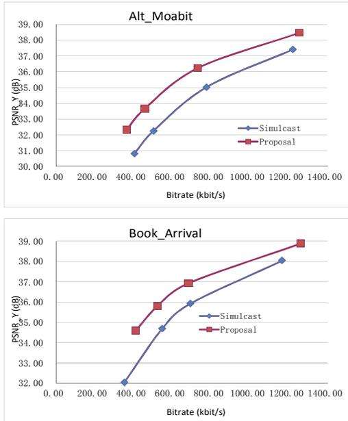
**Fig.7.** RD curve comparisons between simulcast and our proposal
