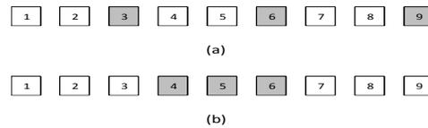
Fig.5. Data loss pattern by the two different cache overflow handling ways (grey packets are lost)
