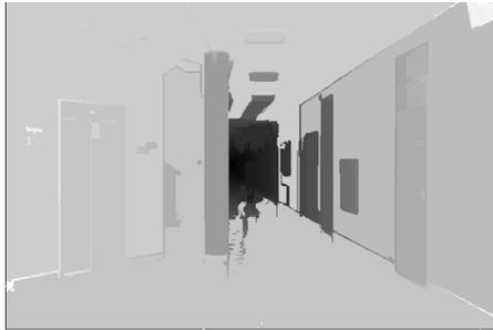
**Fig.4.** Depth map reconstructed by depth template plus objects segmentation
